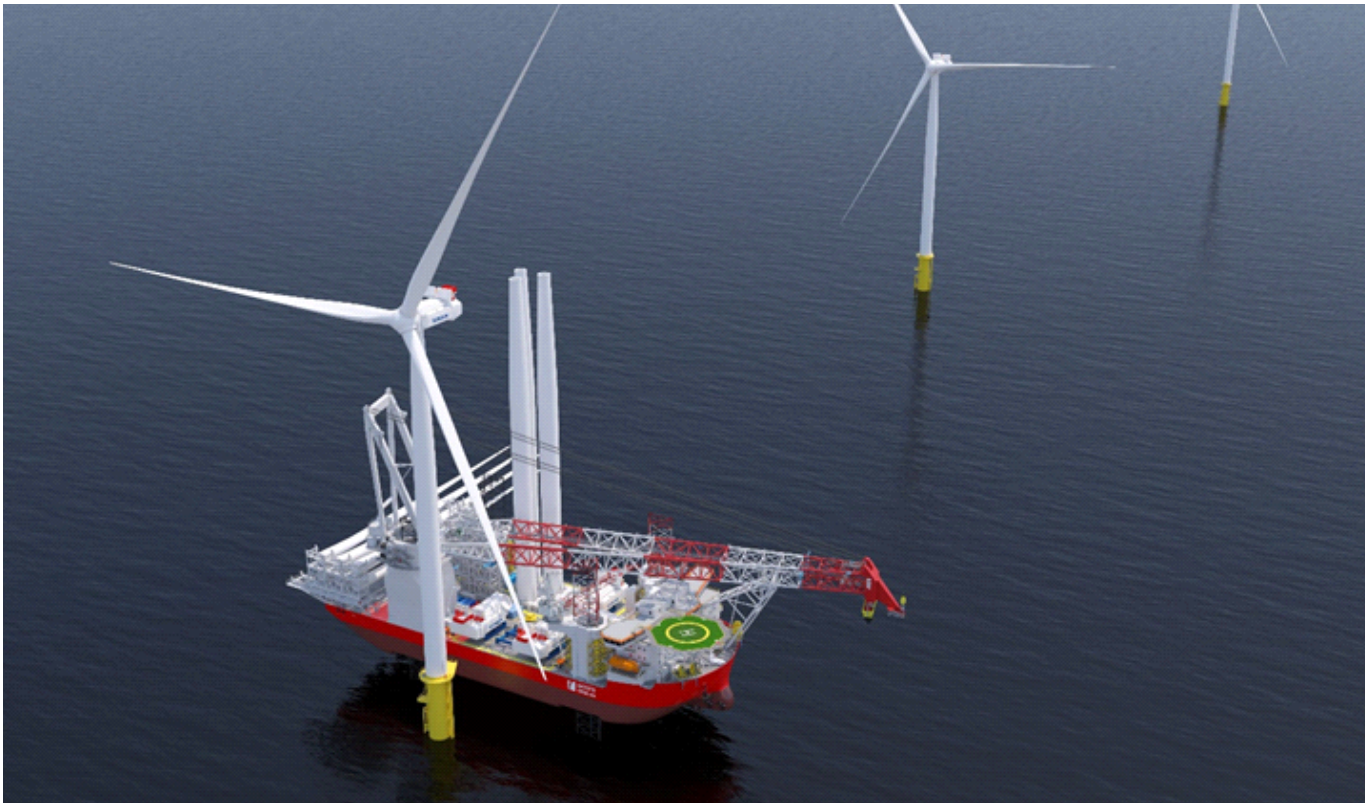
Photo: Illustration of the concept WTIV (Wind Turbine Installation Vessel) during offshore installation.
